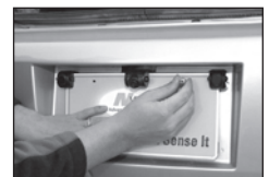
Secure license plate bracket with provided screws
