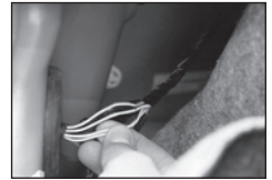
Locate the reverse light wire and splice the red wire to the reverse light wire
